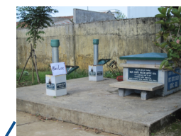
Multiparameter GPRS Data-loggers in the Dong Nai River Basin
